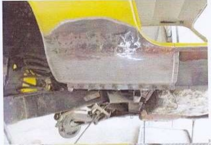
Rusted bottem door frame New made up sill
